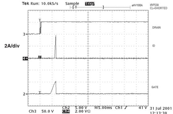
The maximum current that may occur during this period can be controlled by adding a resistor in series with the source of the MOSFET. The lower graph shows the same circuit with a  $100\text{m}\Omega$  resistor inserted between source and  $V_{NN}$ . In this case the maximum current is 25% smaller.
