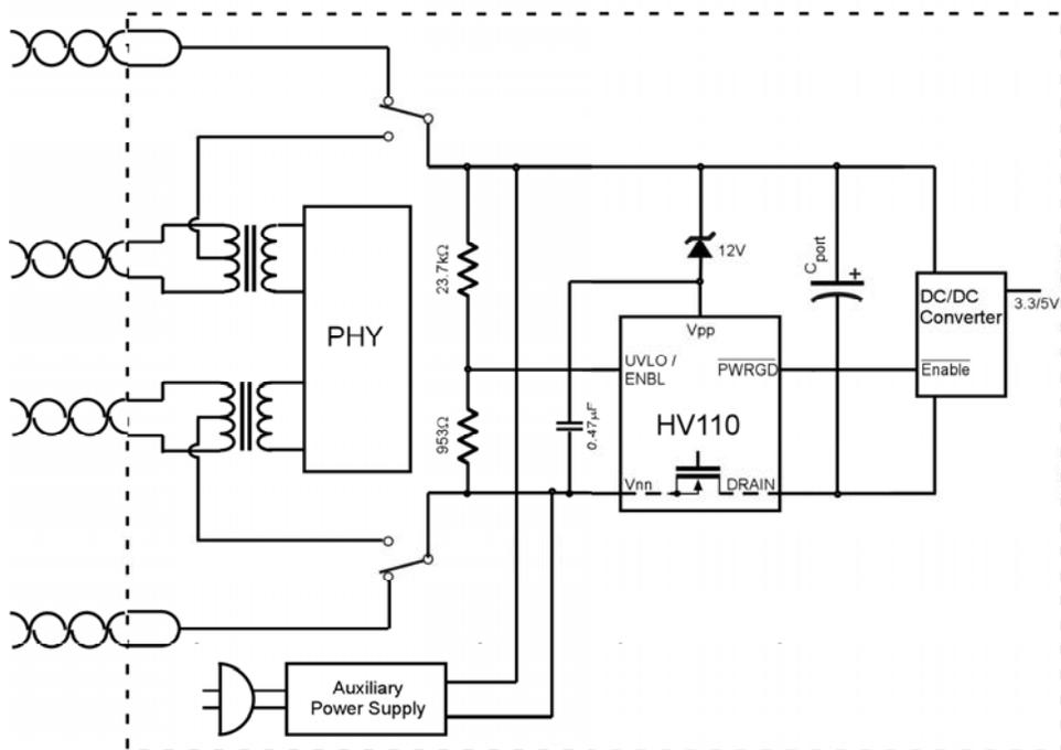
Figure 11. Powering HV110 from an Auxiliary power source
